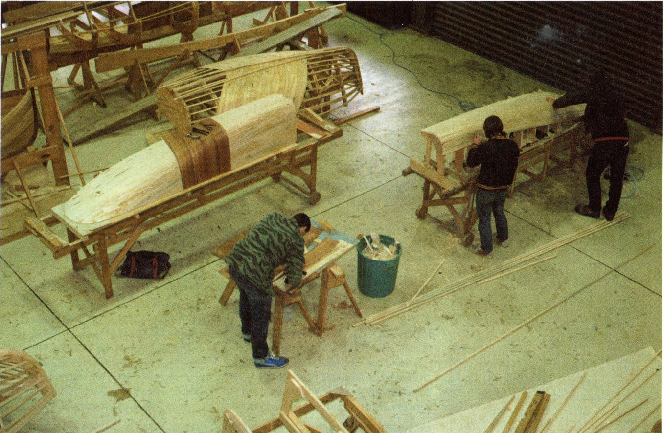
Students building the plugs for the bolt-together canoes made in the FRP shop. (Iain Forsyth collection)
