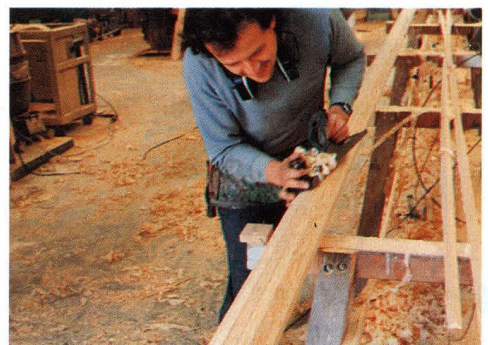
A new mullet boat mast under construction in our workshop.
