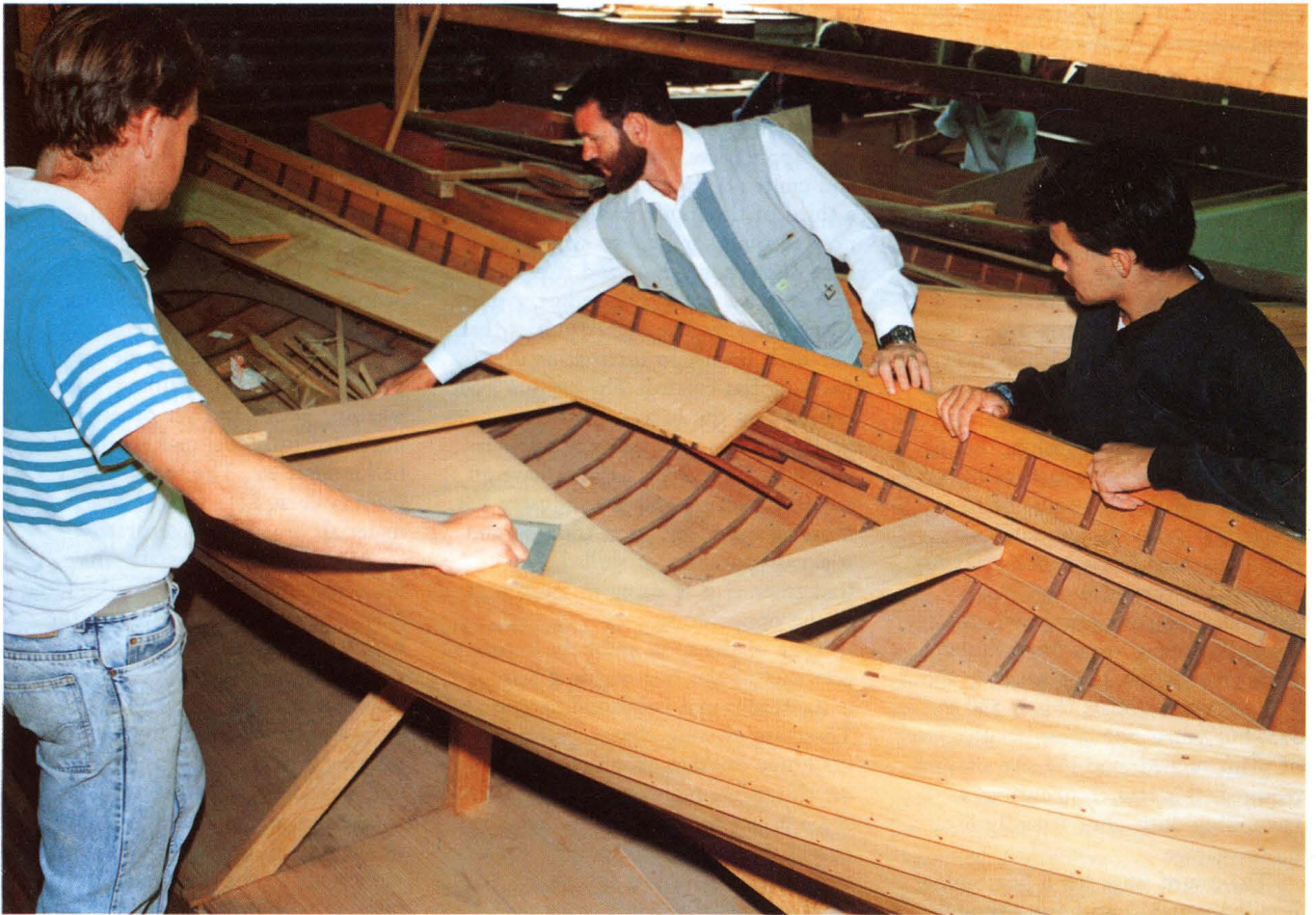
Hulls built by the Traditional Boatbuilding class. Iain Forsyth and students discuss a clinker rowing boat. (Gillian Chaplin)
