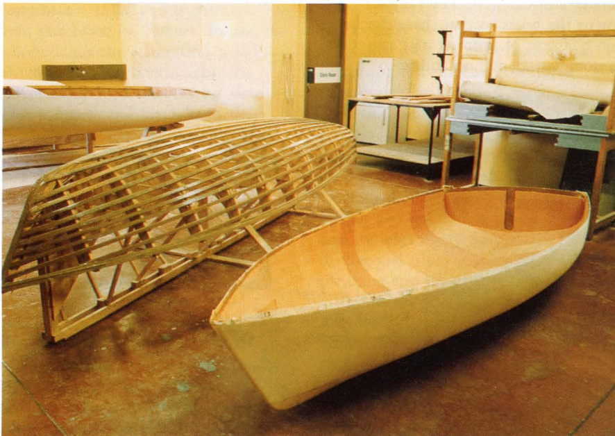
A plug and 'core' constructed 3.5 sailing hull built in 1984. (Iain Forsyth collection)
